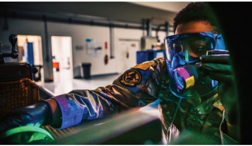
Finding the cracks: A U.S. Air Force non-destructive inspection specialist assigned to the 379th Expeditionary Maintenance Squadron shines a blacklight on a magnetic particle machine within the U.S. Central Command area of responsibility, Dec. 20, 2024. NDI specialists focus on inspecting damages in aircraft equipment and systems unseen by the naked eye. (U.S. Air Force photo by Airman 1st Class Zeeshan Naeem) ◀
